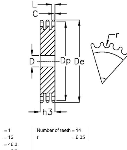
C = 1 D = 12 De = 46.3 Dp = 42.8 For chain size =  $3/8 \times 7/32$ For chain type = 06 B-3 h3 = 25.6 L = 5.2
